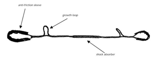
Full Cobra Cable System; Note Anti-Friction Sleeve, Growth Loop, and Shock Absorber. This Support Cable System Allows Natural Flexing of Trees, Stimulating Natural Growth and Strengthening Responses.
