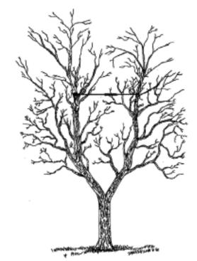
Multiple cables are often recommended to maximize strength; ideally, triangles or boxes should be formed between cabled leads. Cobra cables are providing new options in some cases where trees may have had to be removed in the past.
